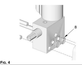
Clean surface of the Dyna-Star pump outlet with a clean dry cloth. Inspect pump surface for scratches or nicks. A scratched surface can result in fluid leakage.
